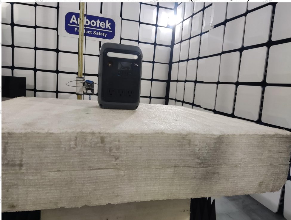
Photo of Radiation Emission Test (above 1GHz)
