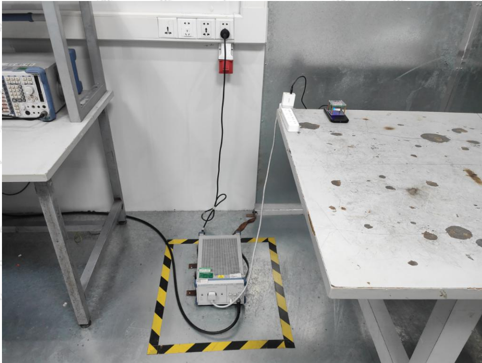
Photo of Conducted Emission Measurement
