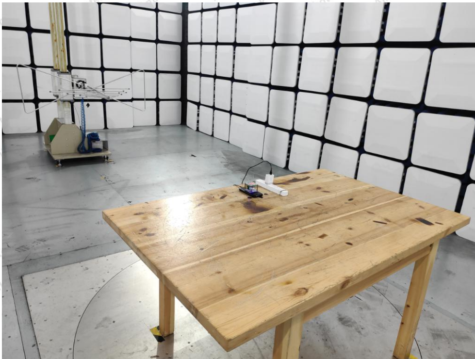
Photo of Radiation Emission Test
