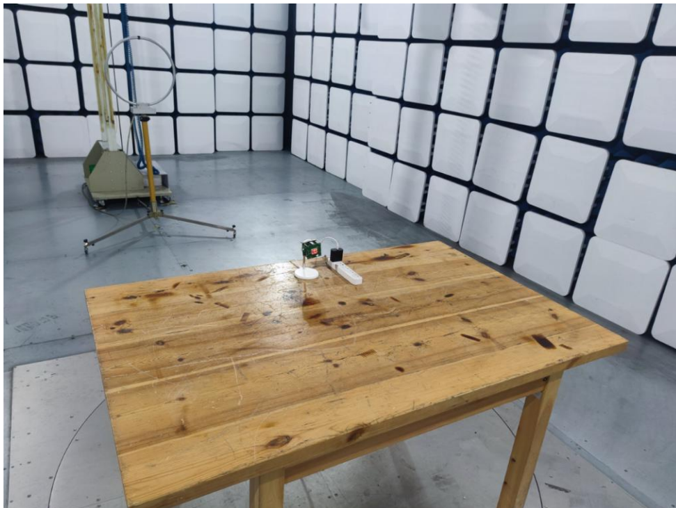
Photo of Radiation Emission Test
