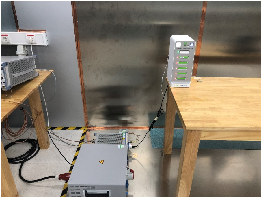
Photograph 3: Set-up for Conducted Emission on AC Mains
