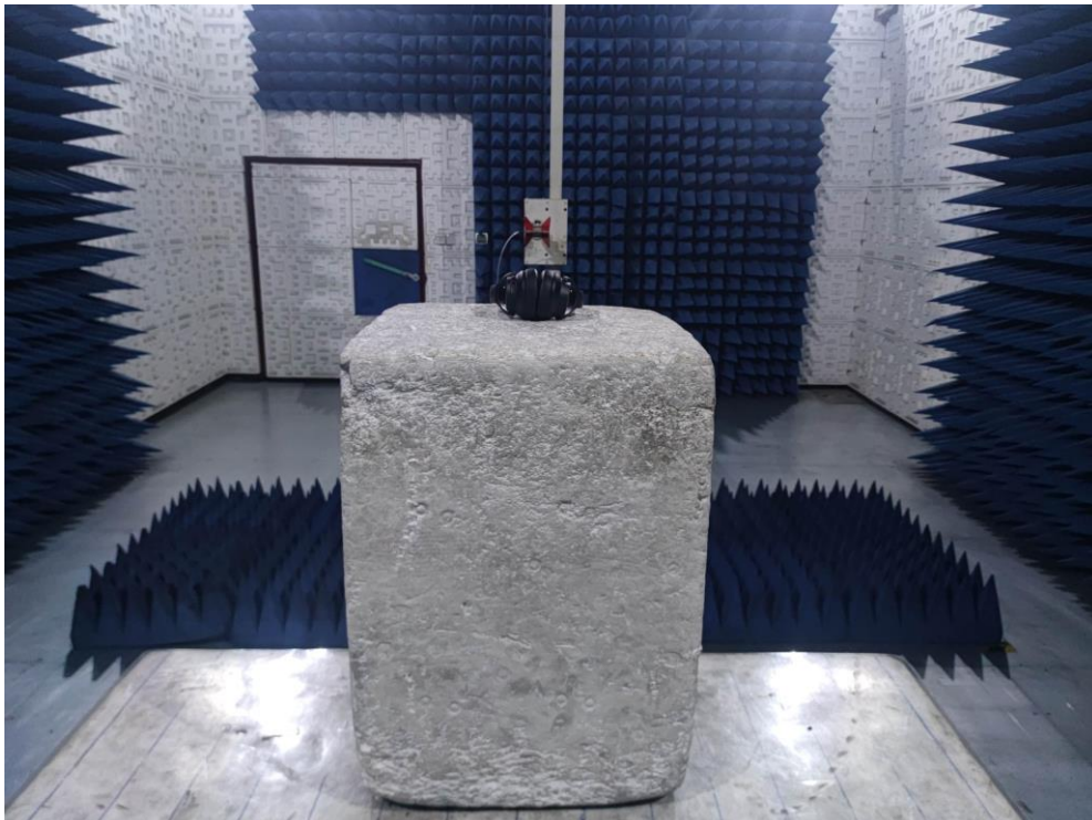
RADIATED EMISSION TEST SETUP ABOVE 1GHz
