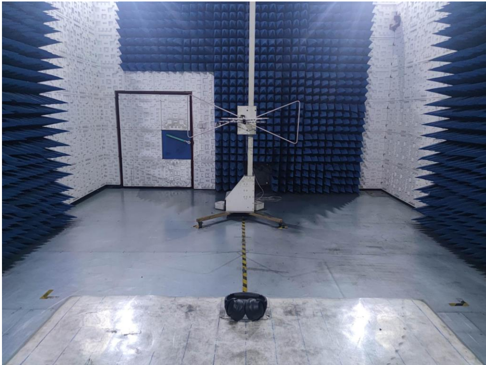
RADIATED EMISSION TEST SETUP ABOVE 1GHz
