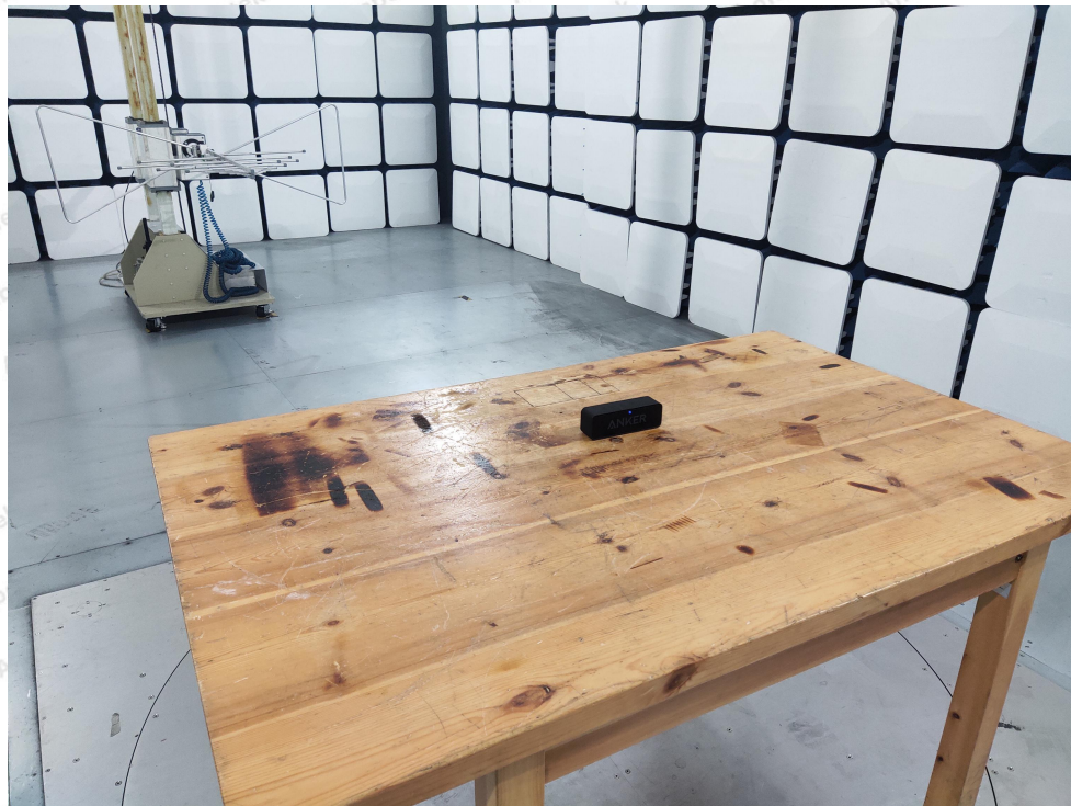
Photo of Radiation Emission Test
