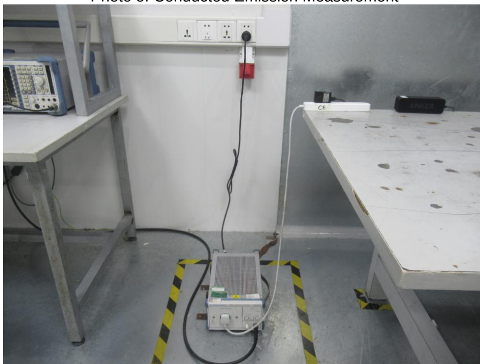
FCC ID: 2AOKB-A3102V Photo of Conducted Emission Measurement
