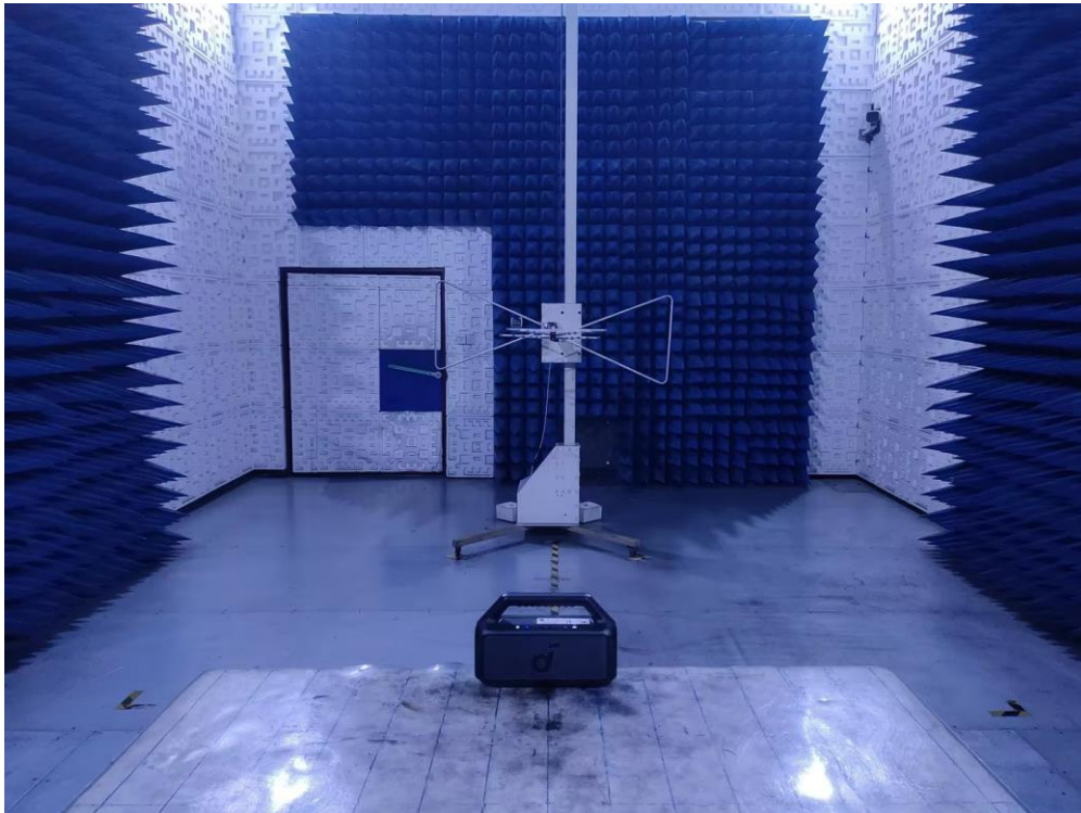
RADIATED EMISSION TEST SETUP ABOVE 1GHz
