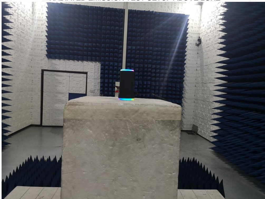
RADIATED EMISSION TEST SETUP ABOVE 1GHZ
