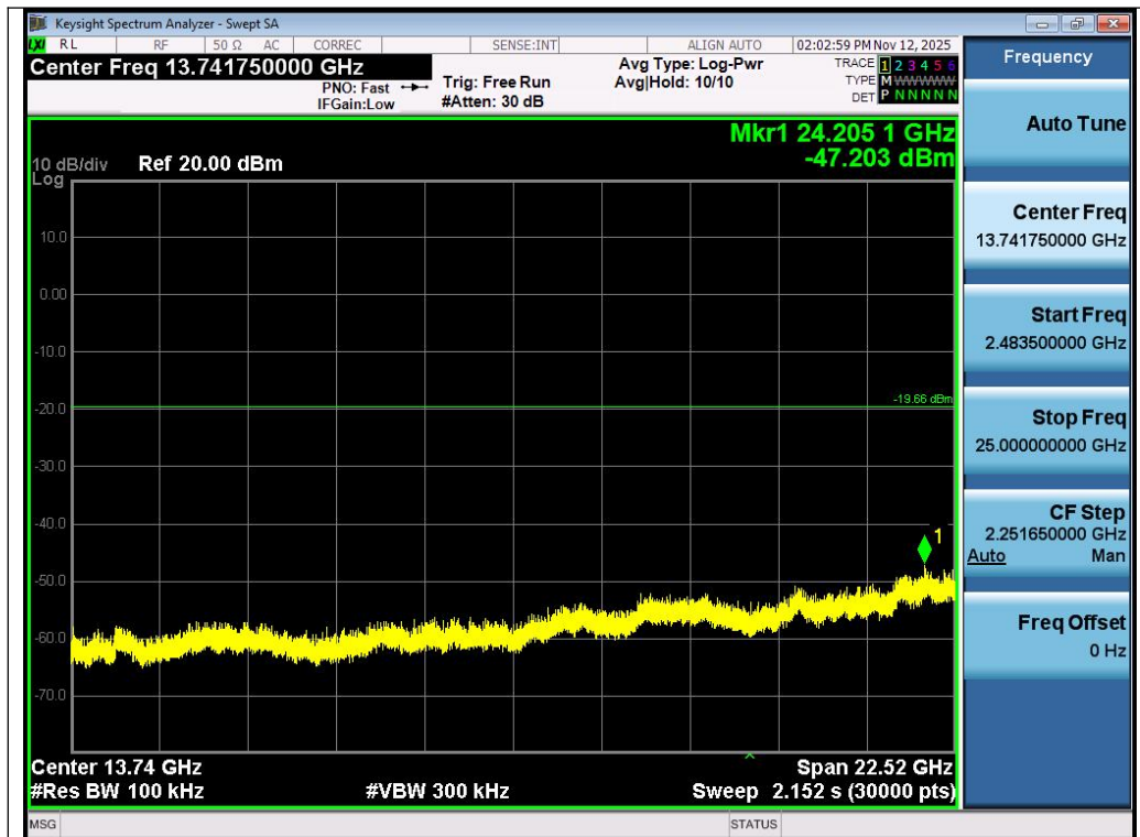
Test_Graph_LE2M_ANT1_2440_2Mbps_Higher Band Emissions
