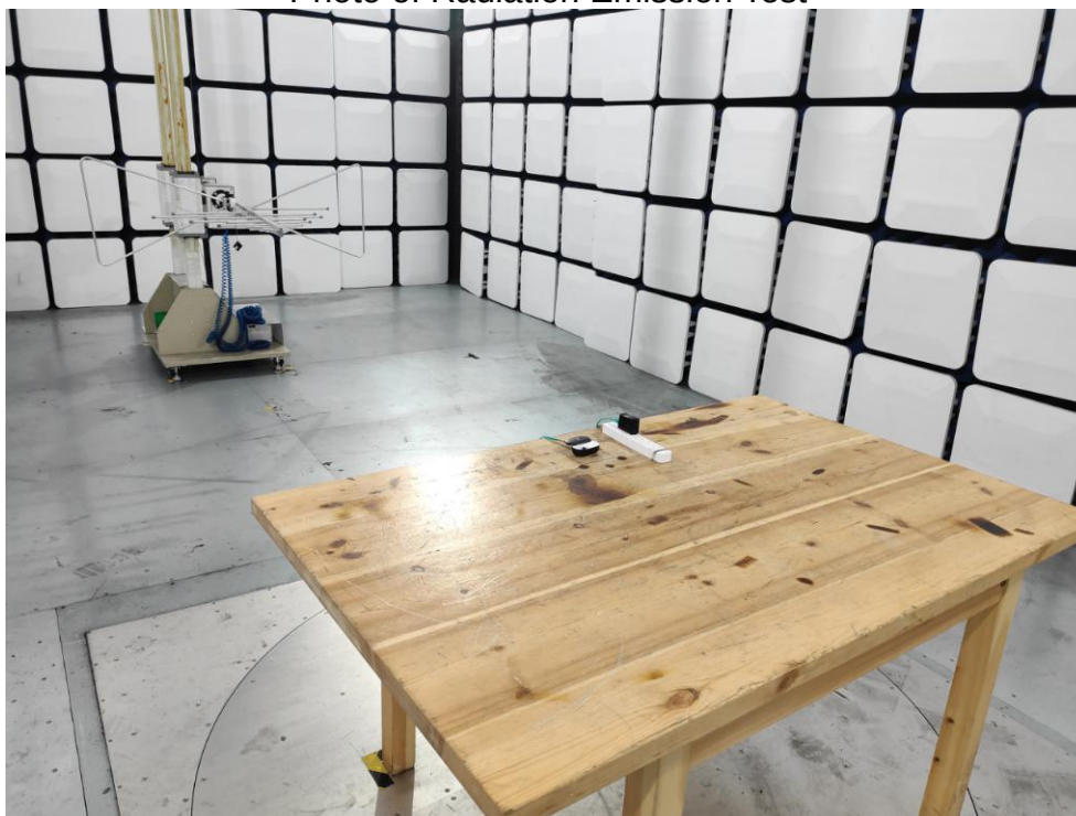
Photo of Radiation Emission Test
