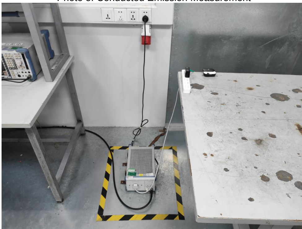
FCC ID: 2AOKB-A3904L Photo of Conducted Emission Measurement
