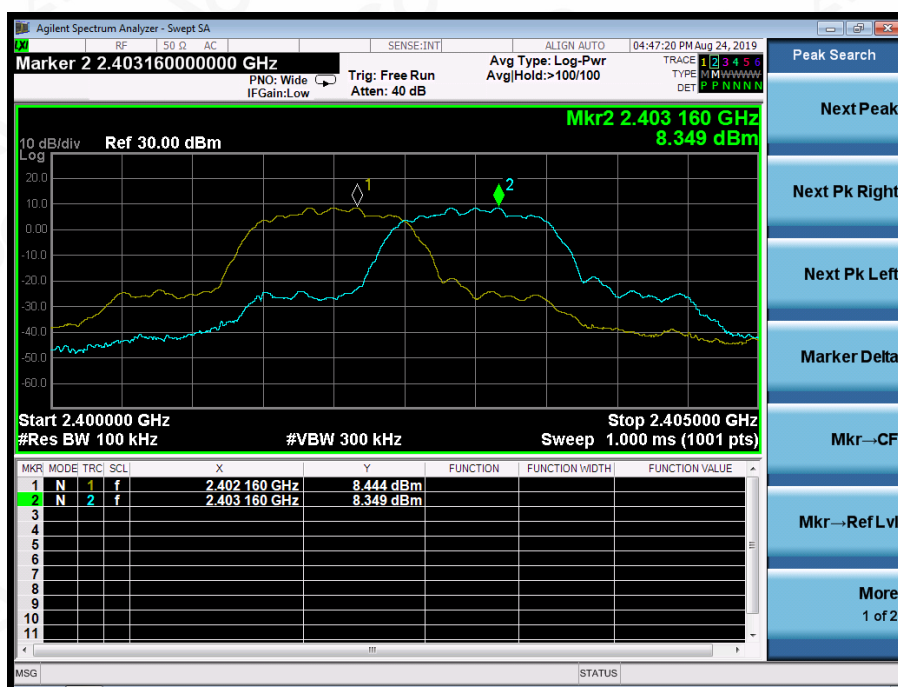
TEST PLOT FOR FREQUENCY SEPARATION
