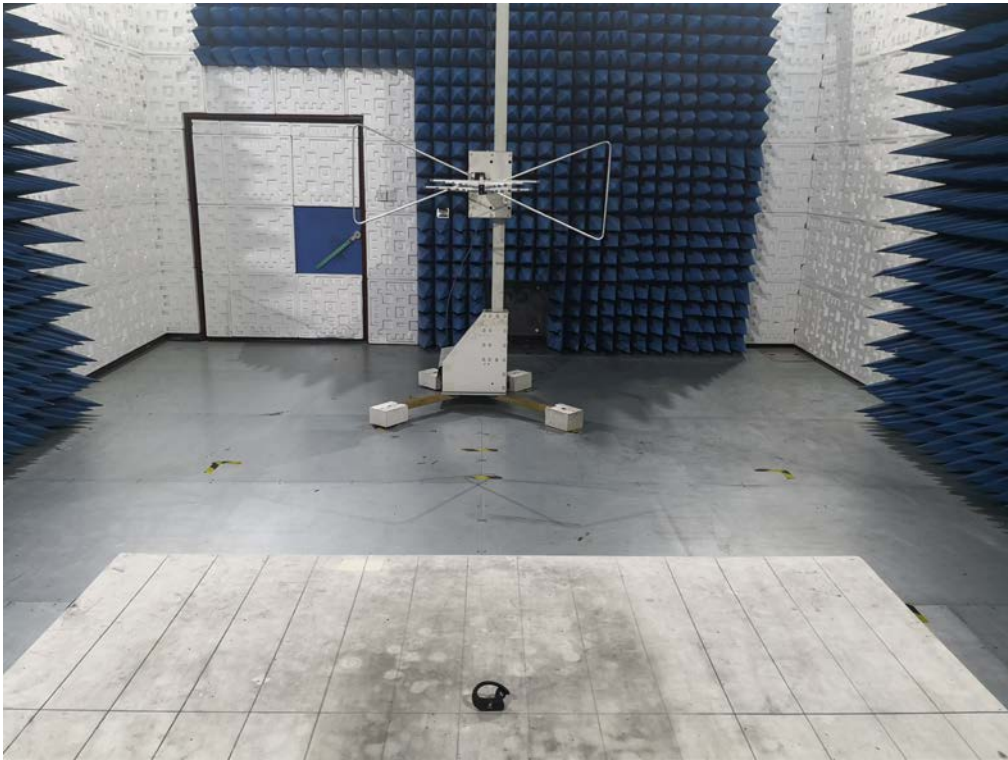
RADIATED EMISSION TEST SETUP ABOVE 1GHZ
