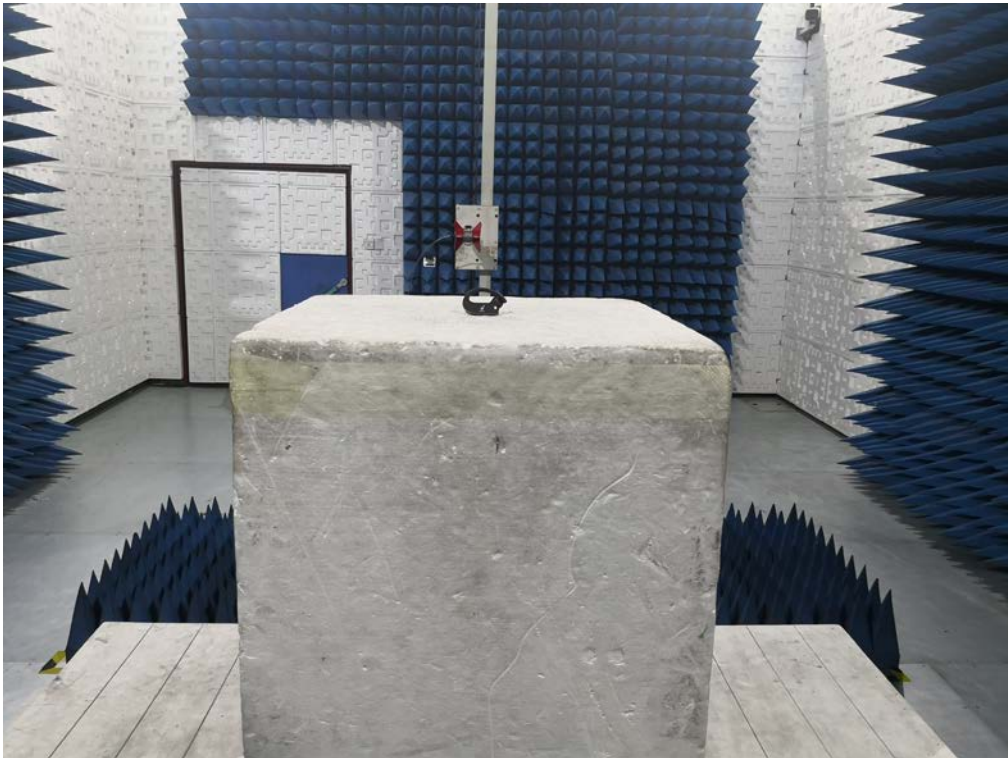
RADIATED EMISSION TEST SETUP ABOVE 1GHZ
