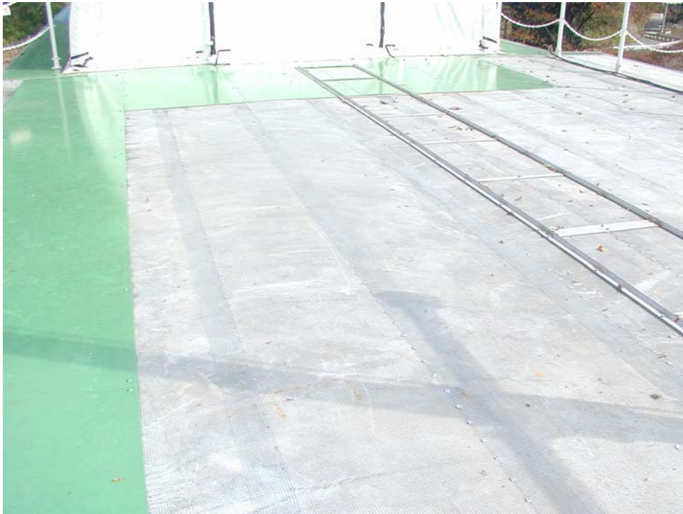
CONDUCTING GROUND PLANE
