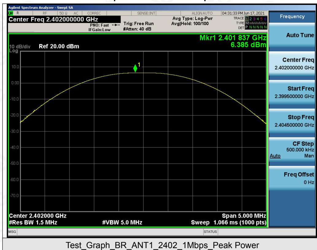
Test Graphs of Conducted Output Power
