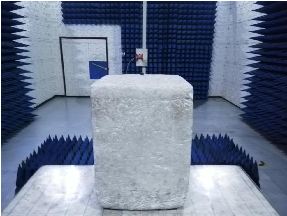
RADIATED EMISSION TEST SETUP ABOVE 1GHz
