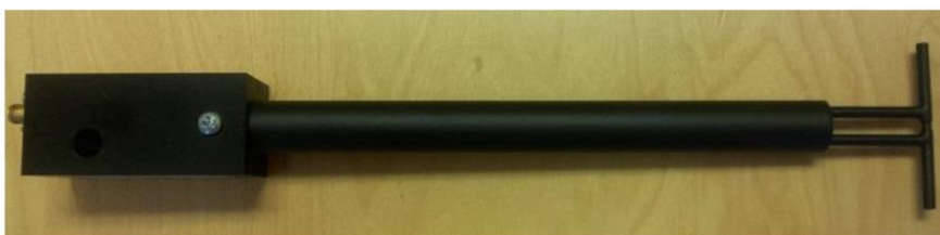
Figure 1 – MVG COMOSAR Validation Dipole
