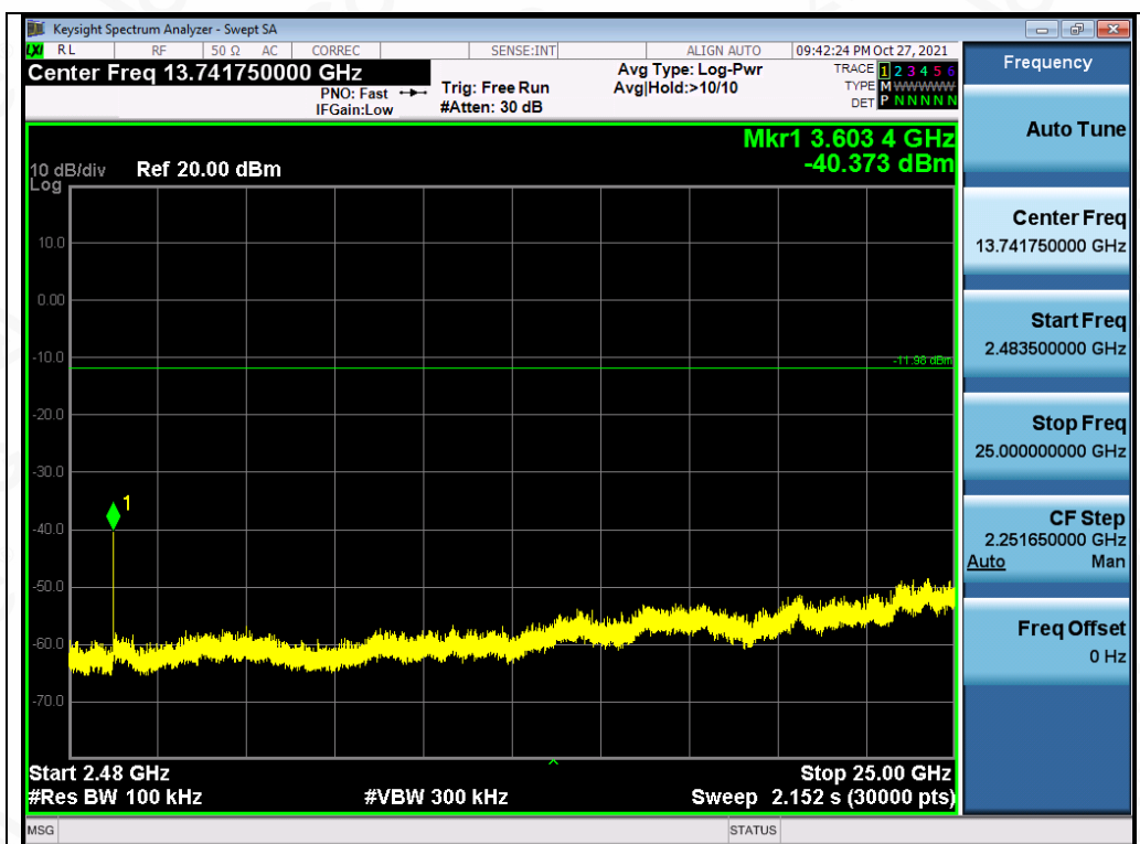
Test_Graph_BR_ANT1_2402_1Mbps_Higher Band Emissions
