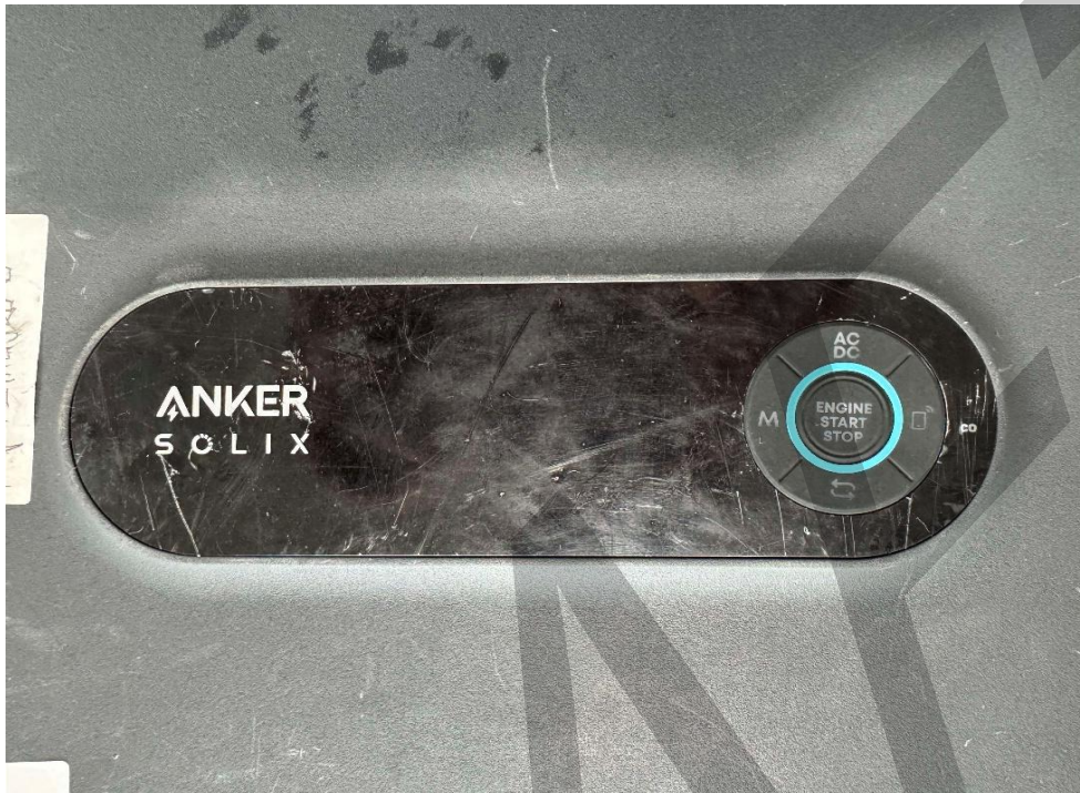
Photo 11 - Control panel in top
