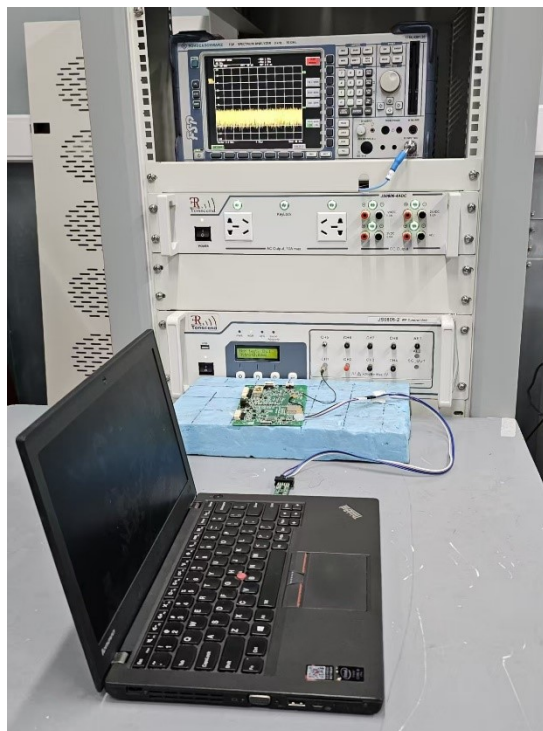
Photograph 4: Set-up for Radio Spectrum Testing
