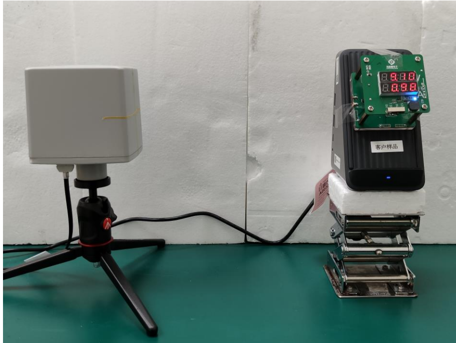
Photograph 8: Set-up for H-field strength (Left View)
