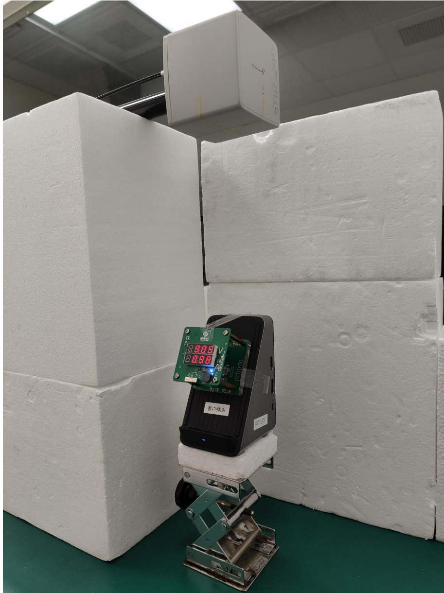
Photograph 10: Set-up for H-field strength (Top View)
