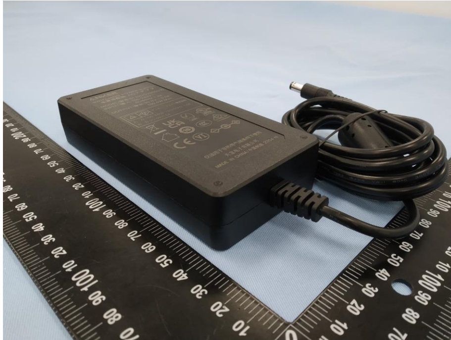
Photograph 13: Support Units (Switching Power Supply)
