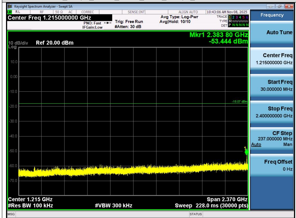
Test_Graph_LE1M_ANT1_2480_1Mbps_Lower Band Emissions
