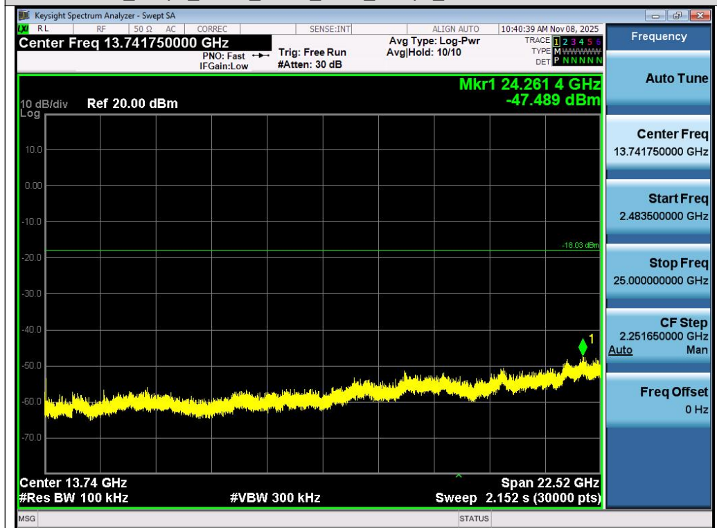
Test_Graph_LE1M_ANT1_2440_1Mbps_Higher Band Emissions
