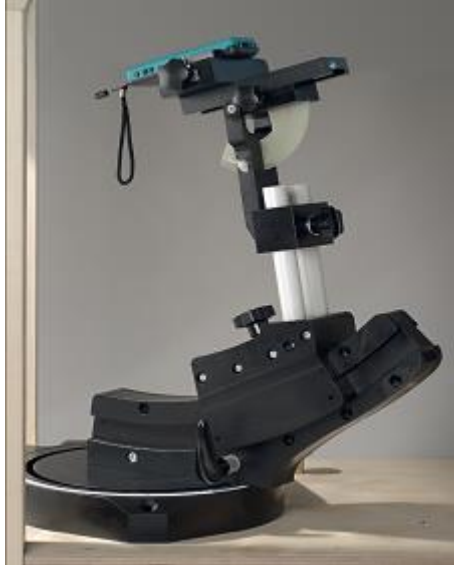
F-2. Device Holder for Transmitters
