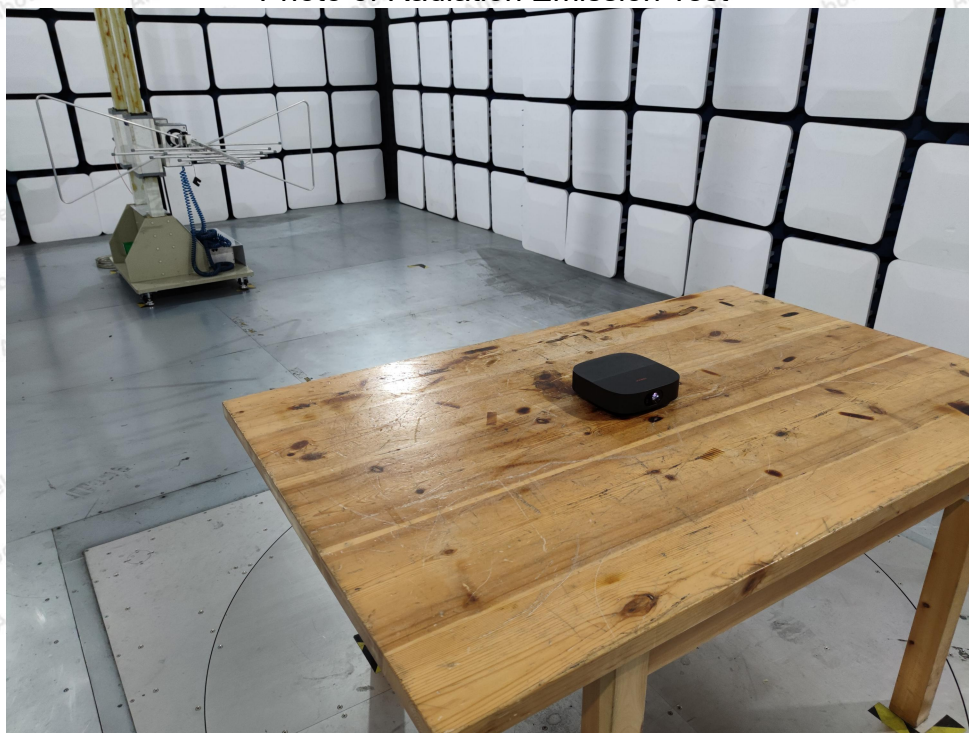
Photo of Radiation Emission Test
