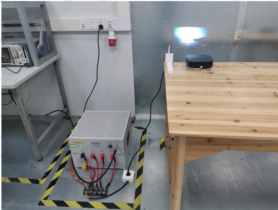
Photo of Conducted Emission Measurement
