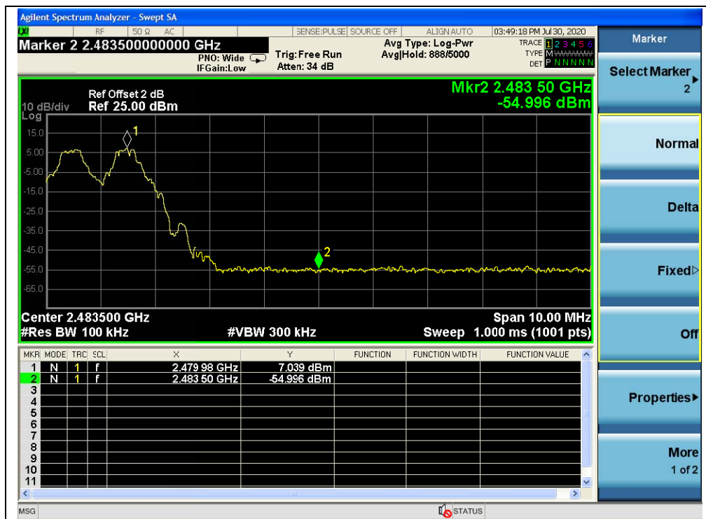
(Band edge with hopping on, Channel 78, GFSK)
