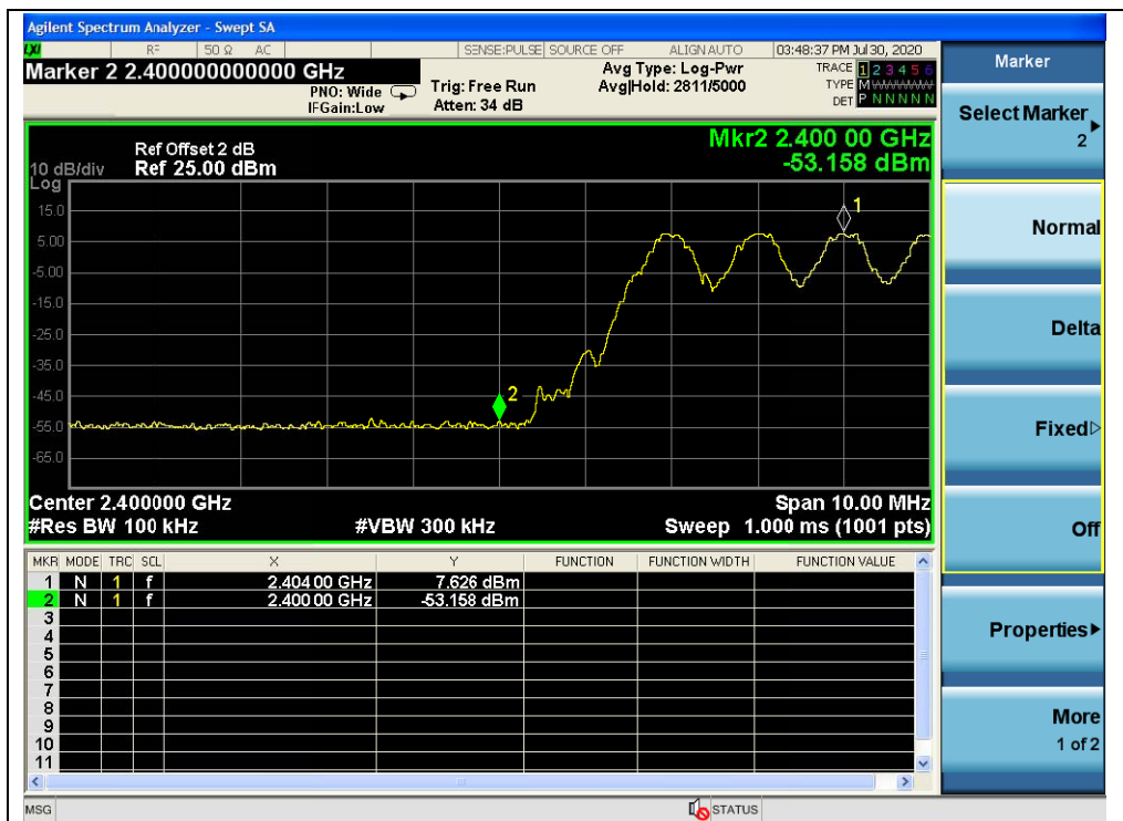
(Band edge with hopping on, Channel 0, GFSK)
