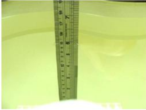
Fig 6.1 Photo of Liquid Height for Head SAR
