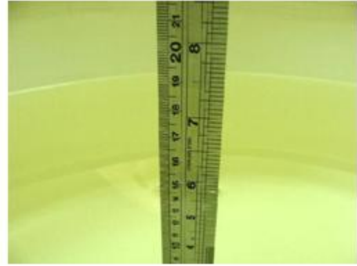
Fig 6.2 Photo of Liquid Height for Body SAR
