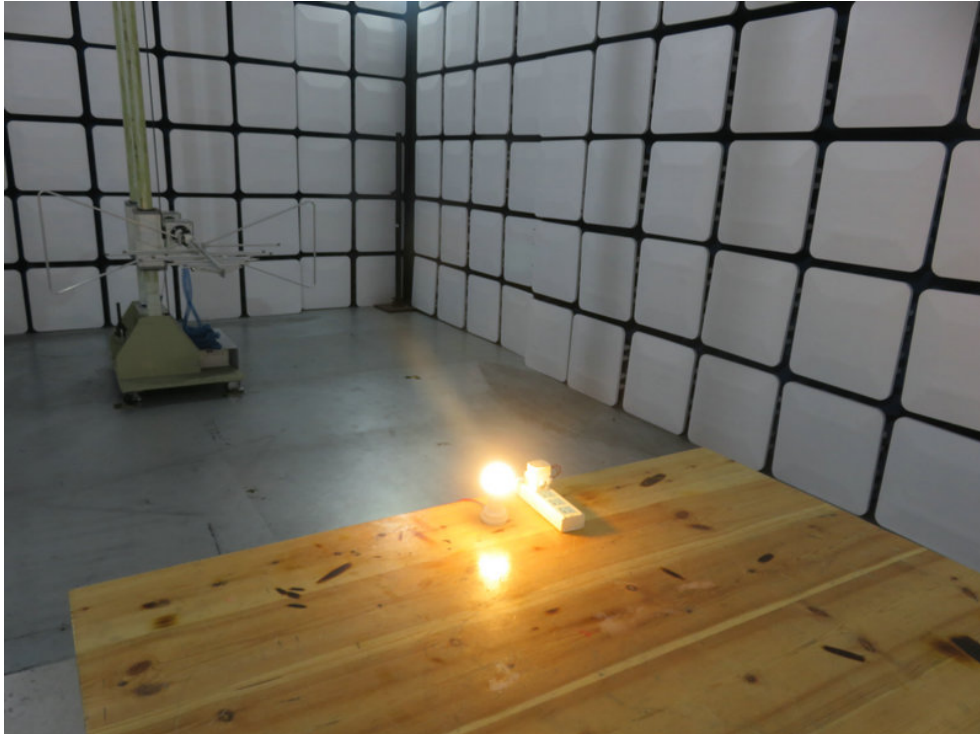
Photo of Radiation Emission Test
