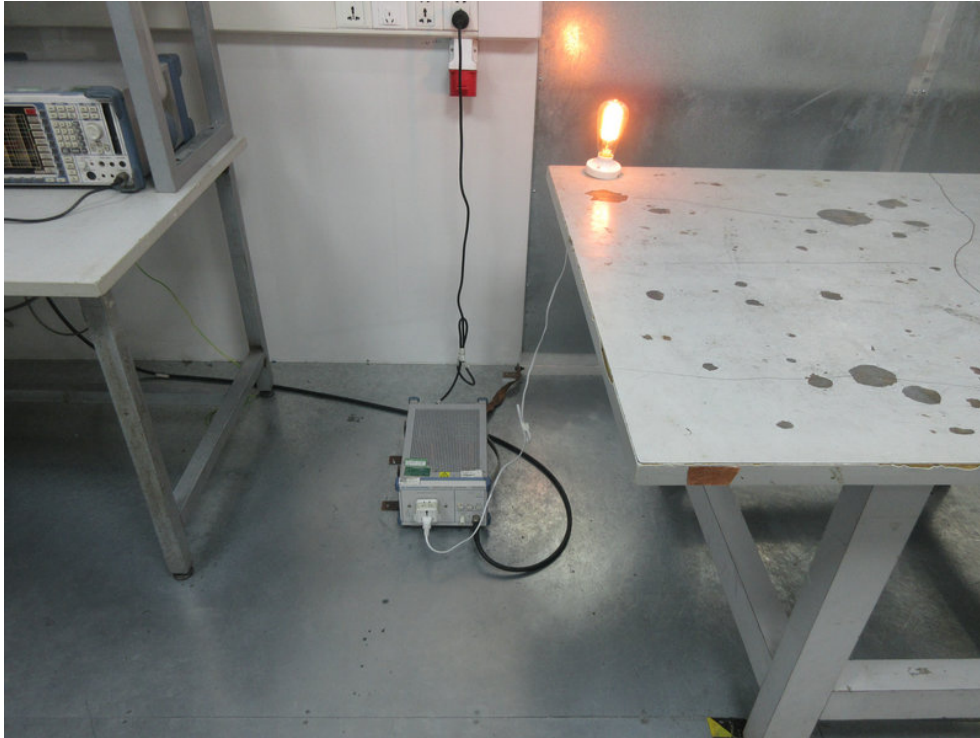
Photo of Conducted Emission Measurement
