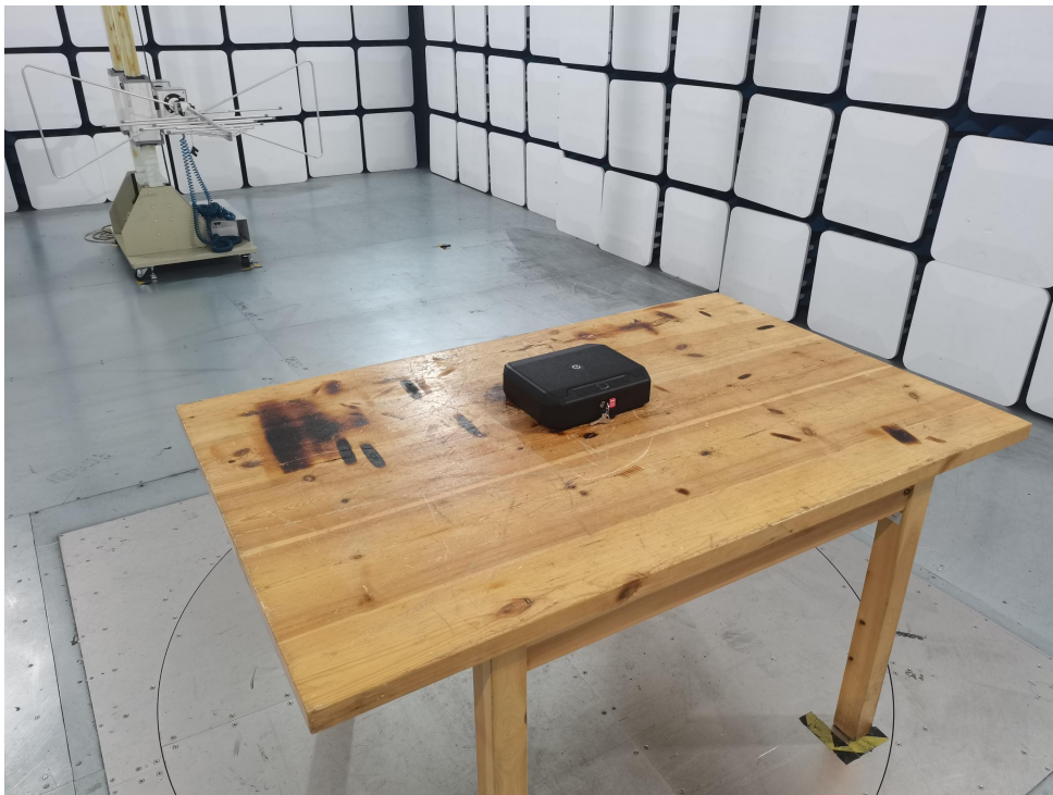
Photo of Radiation Emission Test
