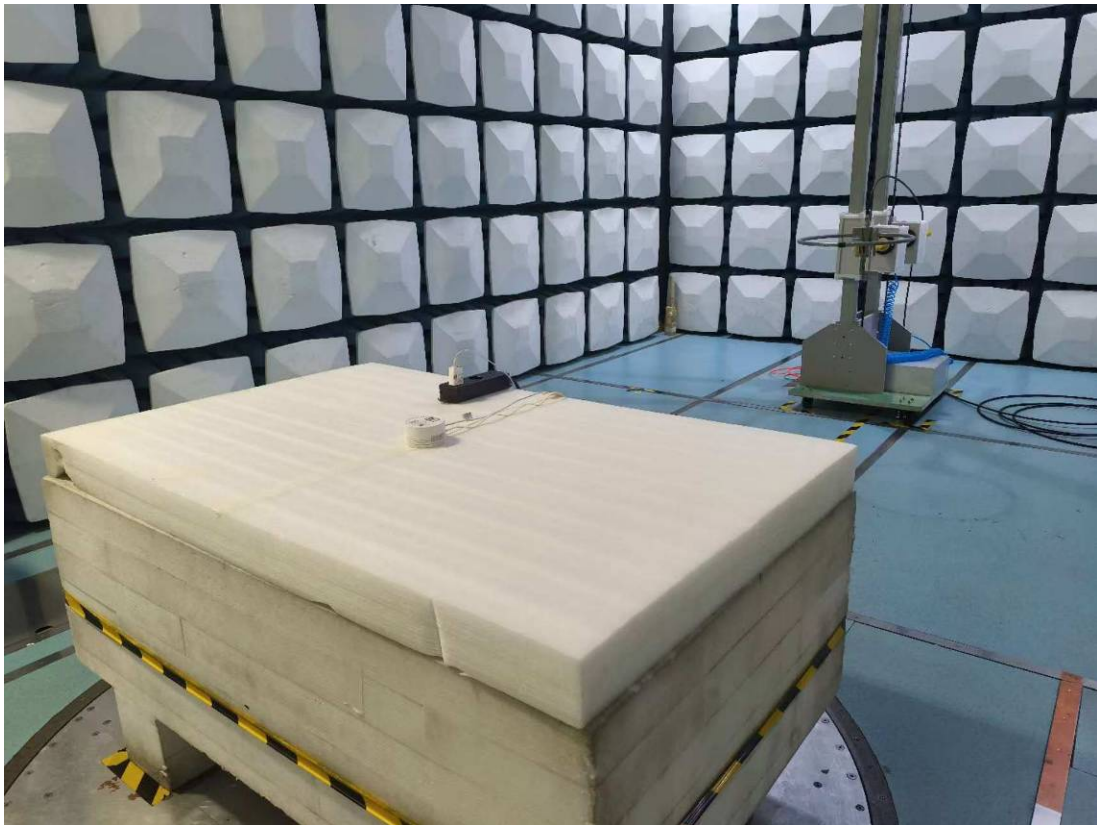
Radiated Emission 30M-1GHz View
