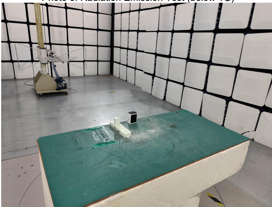
Photo of Radiation Emission Test (below 1G)
