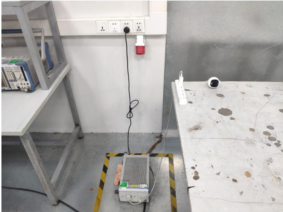
FCC ID: 2AOKB-T8441 Photo of Power Line Conducted Emission Test
