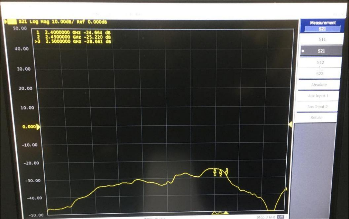
WiFi and BT antenna isolation data (about - 24~- 28dB)
