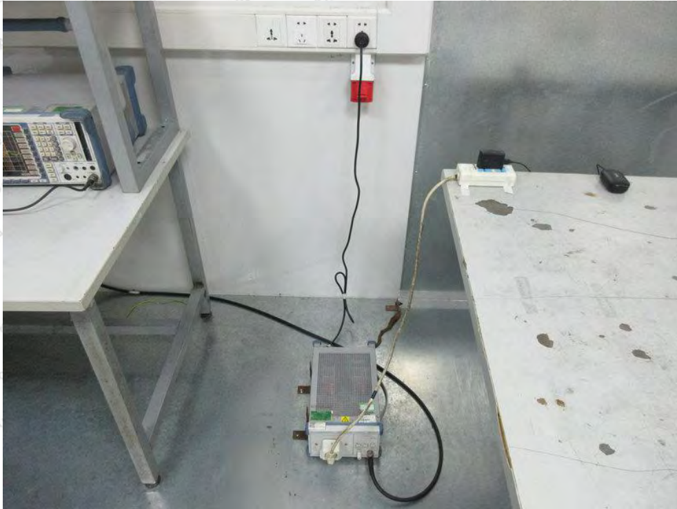
Photo of Conducted Emission Measurement
