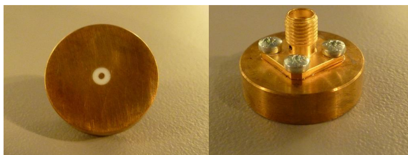
Figure 1 – MVG LIMESAR Dielectric Probe
