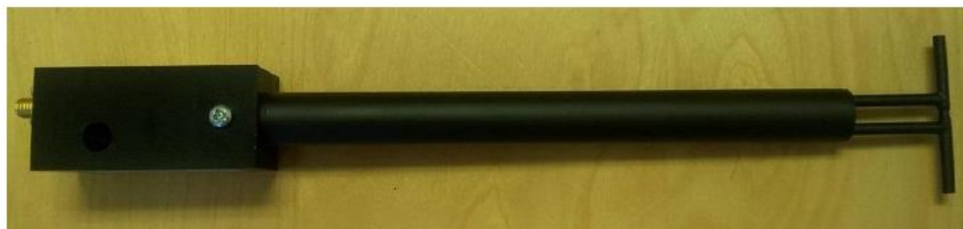
Figure 1 – MVG COMOSAR Validation Dipole
