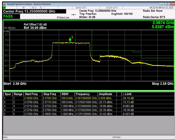
n7 SCS=15kHz DFT_BPSK BW=5MHz HighChannel=513500 RB=25@0
