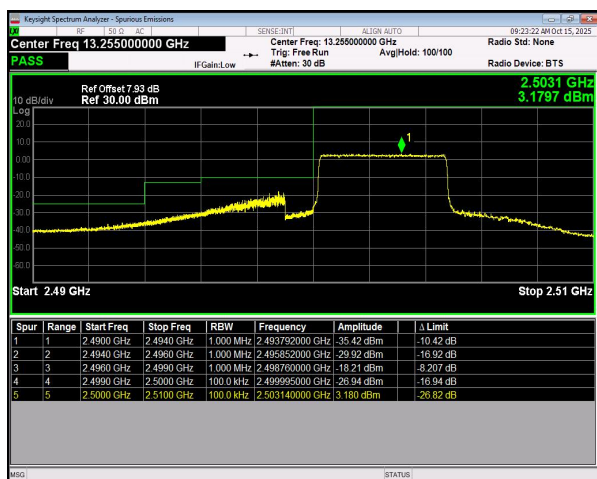
n7 SCS=15kHz CP_QPSK BW=5MHz LowChannel=500500 RB=25@0
