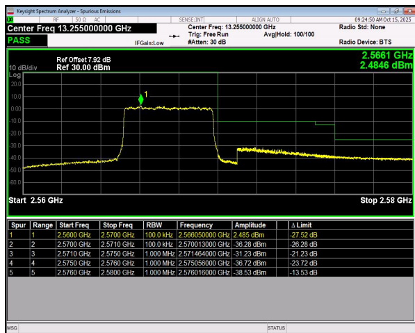
n7 SCS=15kHz DFT_256QAM BW=5MHz HighChannel=513500 RB=25@0
