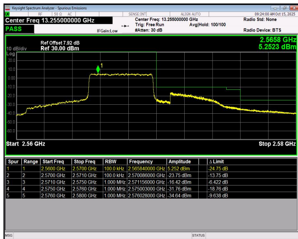
n7 SCS=15kHz DFT_QPSK BW=5MHz HighChannel=513500 RB=25@0
