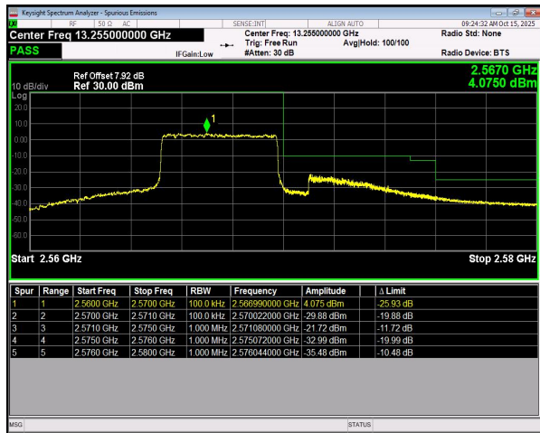
n7 SCS=15kHz DFT_64QAM BW=5MHz HighChannel=513500 RB=25@0
