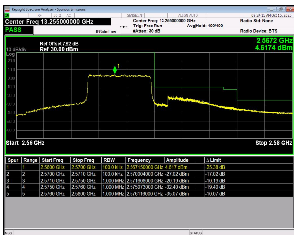
n7 SCS=15kHz DFT_16QAM BW=5MHz HighChannel=513500 RB=25@0
