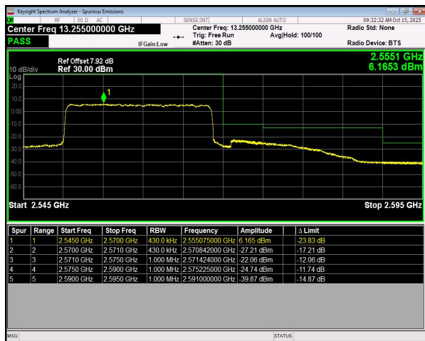
n7 SCS=15kHz DFT_QPSK BW=20MHz HighChannel=512000 RB=100@0
