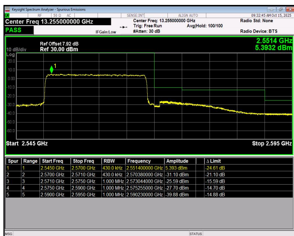
n7 SCS=15kHz DFT_16QAM BW=20MHz HighChannel=512000 RB=100@0
