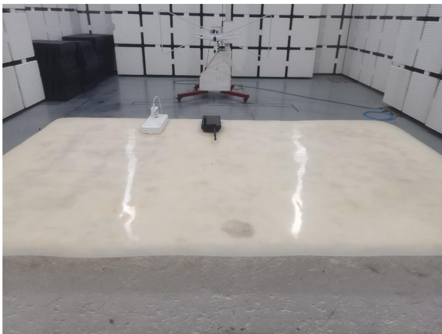
Set-up for Radiated Emission (RE), Below 1GHz
