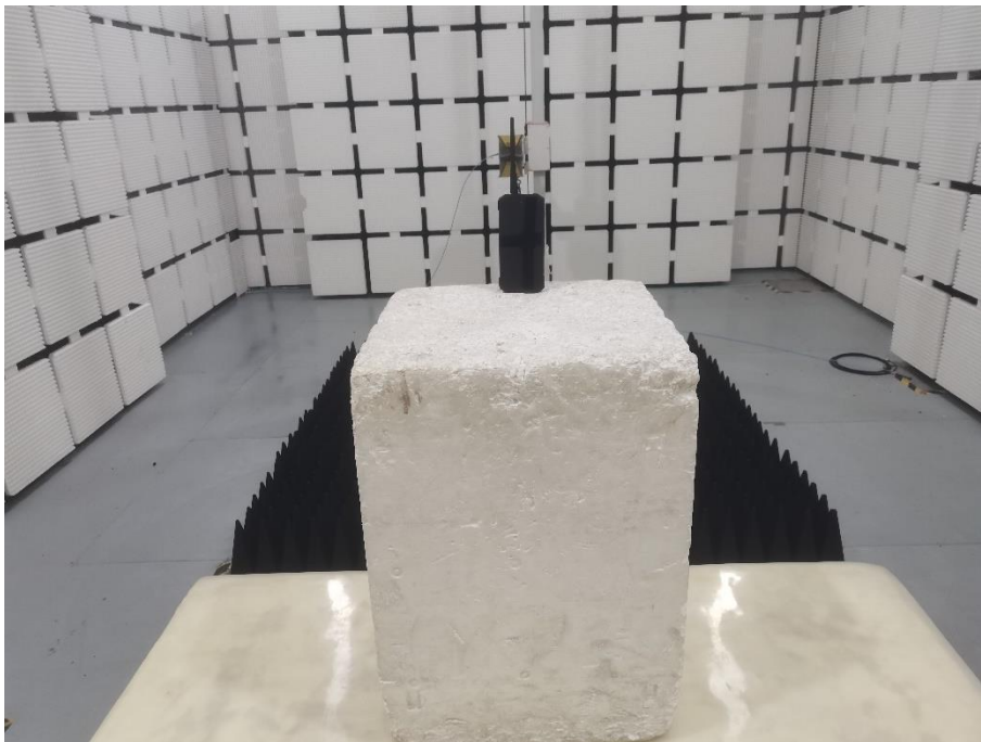
Set-up for Radiated Spurious Emission, Above 1GHz
