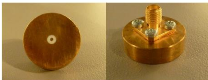
Figure 1 – MVG LIMESAR Dielectric Probe
