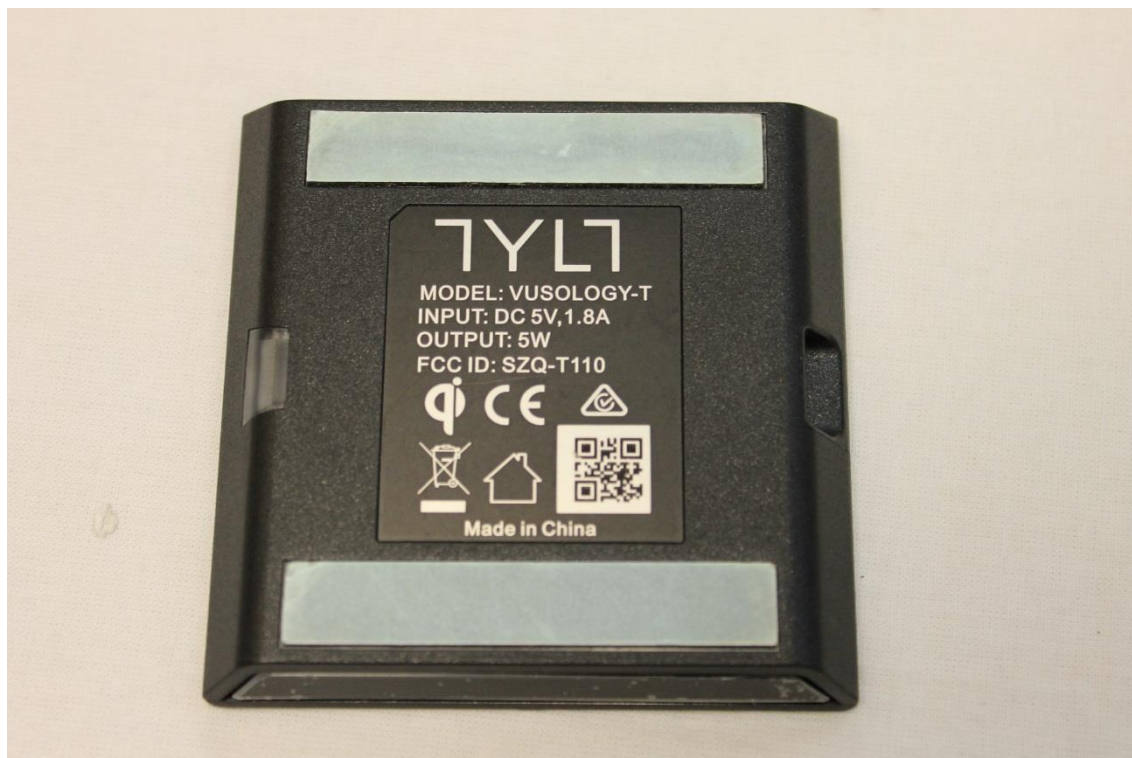
Photograph 3. Wireless charging unit
