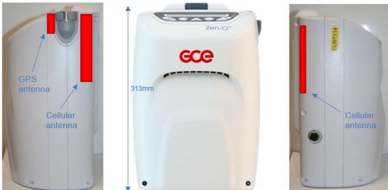
The location of the antenna
