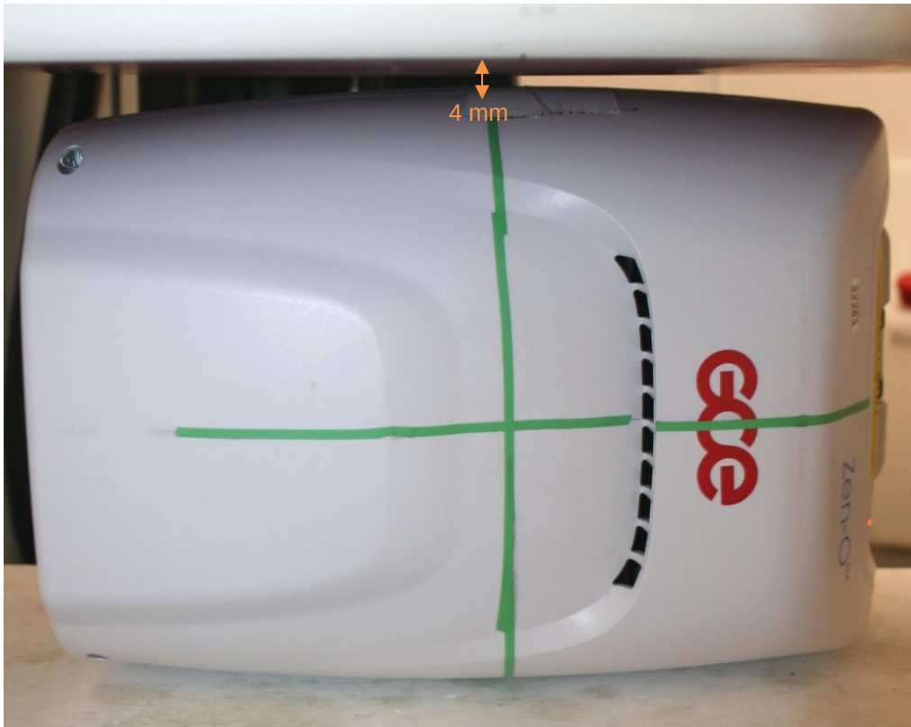
Left side of the device against the phantom, 4mm separation
