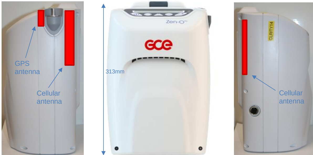
Figure 2 The drawing of the location of the antenna
