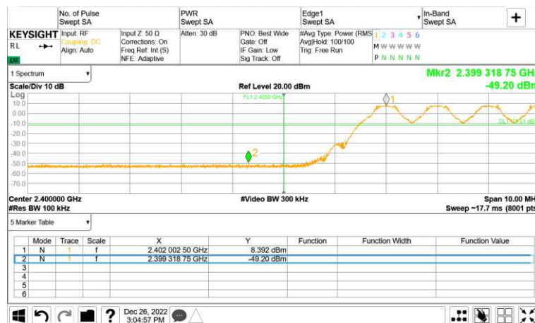
Left, Band Edge, Hopping mode, GFSK, Lowest Channel (2 402 MHz)
