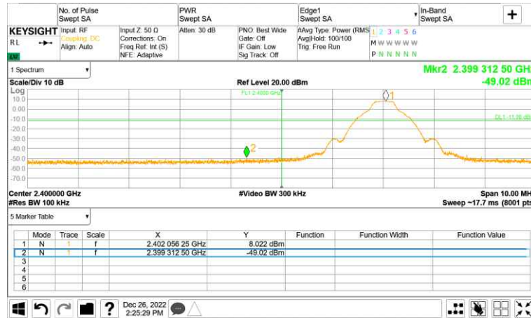
Left, Band Edge, GFSK, Lowest Channel (2 402 MHz)
