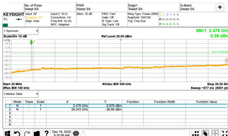
Right, Conducted Spurious Emissions, \pi/4 DQPSK, Highest Channel (2 480 MHz)
