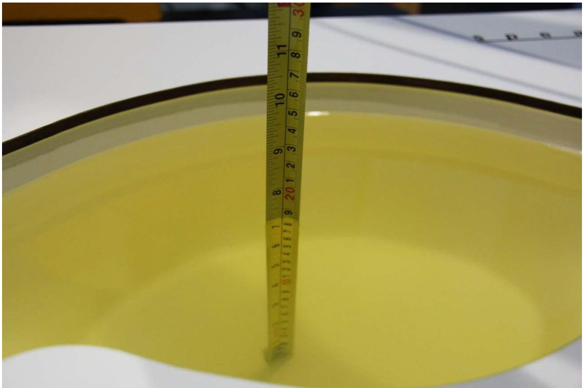
Picture 7-1: Liquid depth in the Flat Phantom(2450MHz)
