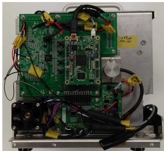
Left side (FPGA, Motor cont. & ADcon)
