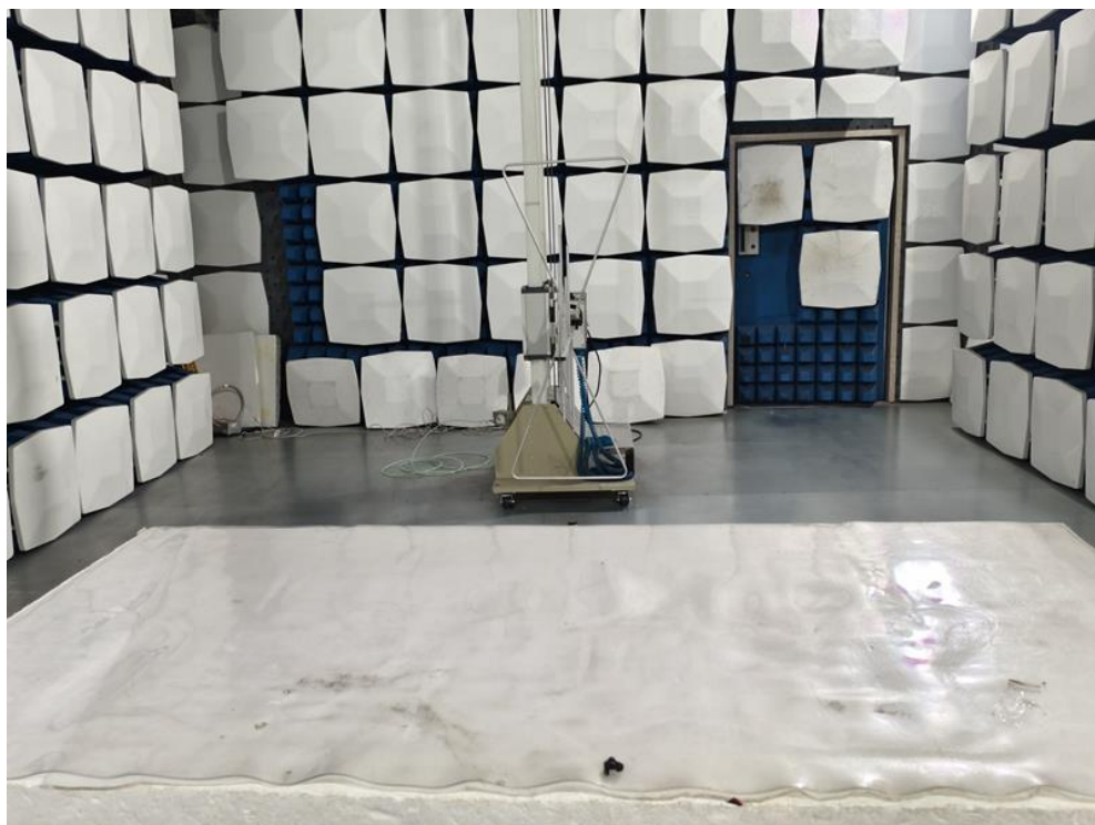
Radiated Emission Test Setup:
