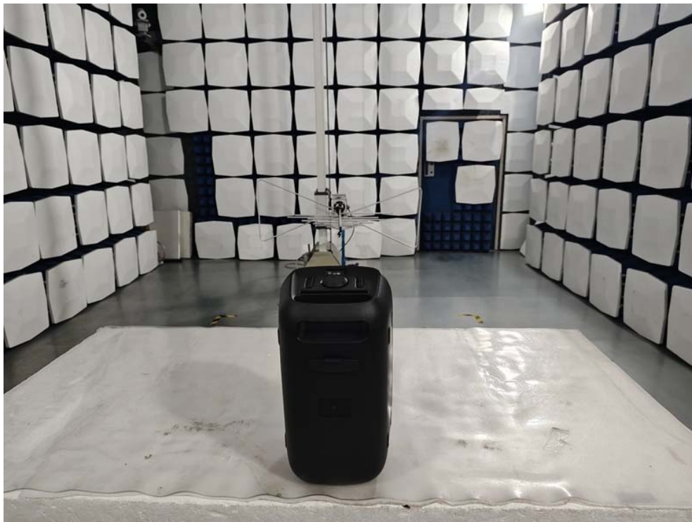
Radiated emission test view
