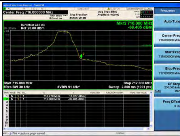
Band12 / 1.4MHz / High CH / QPSK / 1 RB
