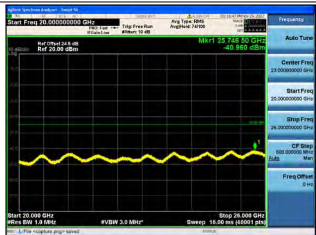
Band7-20G-26G / 20MHz / Low CH / 64QAM
