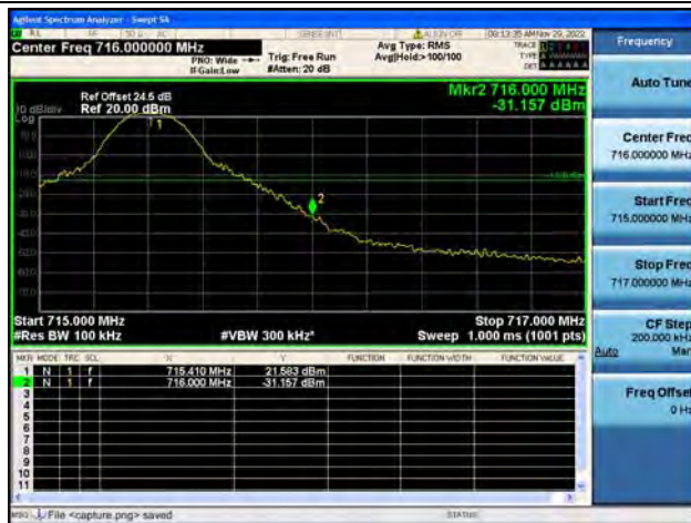
Band12 / 10MHz / High CH / QPSK / 1 RB
