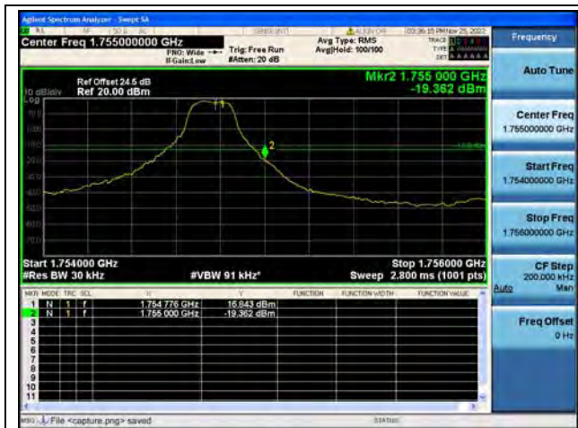
Band4 / 3MHz / High CH / QPSK / 1 RB
