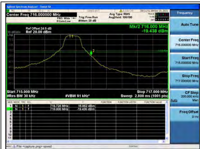
Band12 / 3MHz / High CH / QPSK / 1 RB
