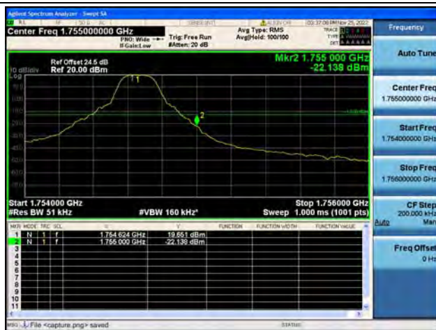
Band4 / 5MHz / High CH / QPSK / 1 RB
