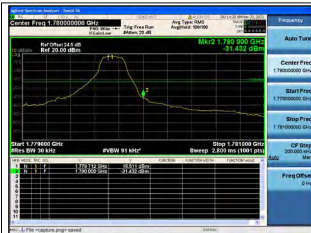
Band66 / 1.4MHz / High CH / QPSK / 1 RB
