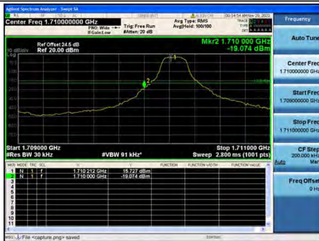
Band66 / 3MHz / Low CH / QPSK / 1 RB
