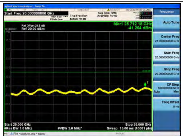
Band7-20G-26G / 15MHz / Mid CH / QPSK
