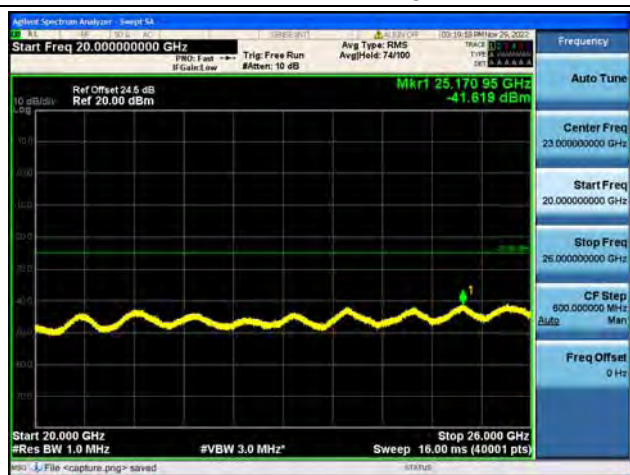
Band7-20G-26G / 20MHz / High CH / 64QAM
