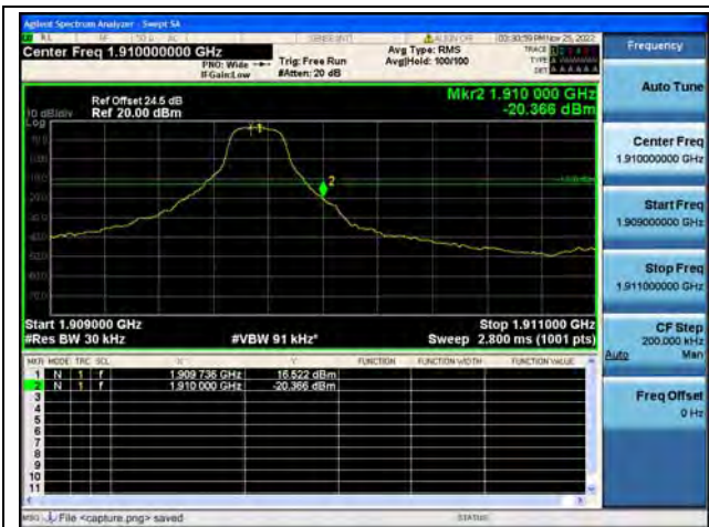
Band2 / 3MHz / High CH / QPSK / 1 RB
