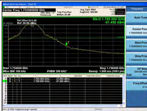
Band4 / 10MHz / High CH / QPSK / 1 RB
