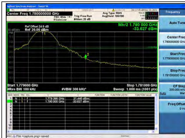
Band66 / 10MHz / High CH / QPSK / 1 RB
