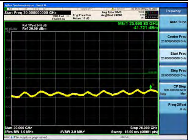
Band7-20G-26G / 15MHz / High CH / 16QAM
