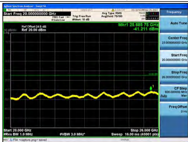
Band7-20G-26G / 20MHz / High CH / 16QAM
