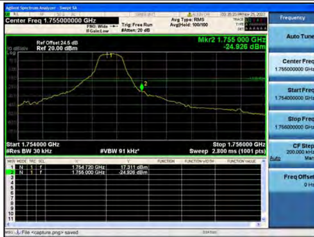
Band4 / 1.4MHz / High CH / QPSK / 1 RB
