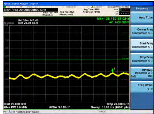
Band7-20G-26G / 20MHz / Low CH / 16QAM
