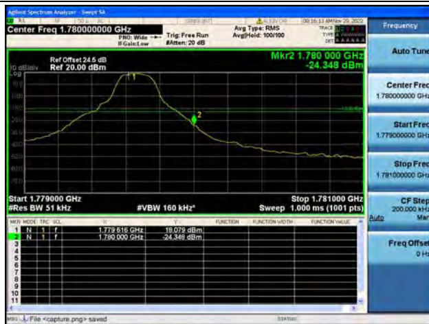
Band66 / 5MHz / High CH / QPSK / 1 RB
