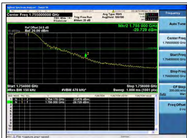
Band4 / 15MHz / High CH / QPSK / 1 RB
