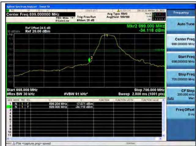
Band12 / 1.4MHz / Low CH / QPSK / 1 RB
