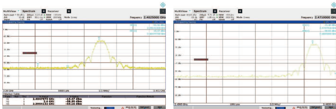
Figure 8: Radiated Emissions at Band Edge, Spectral Diagram, Modes A (2405MHz) and C (2480MHz)
