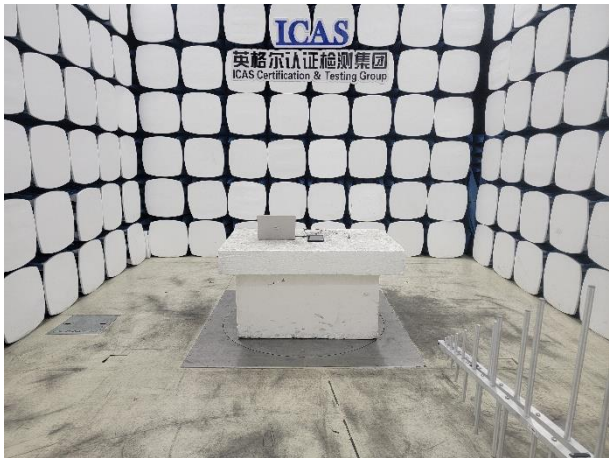
Radiated Emission test set-up for 30M-1GHz, TM133
