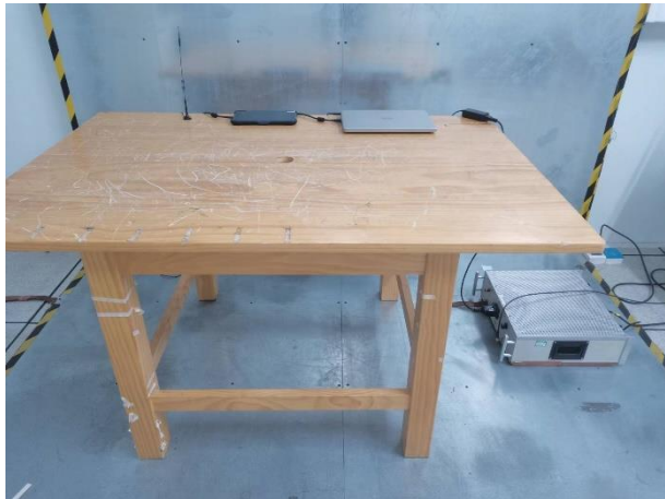
Radiated Emission test set-up for above 1GHz, TM1
