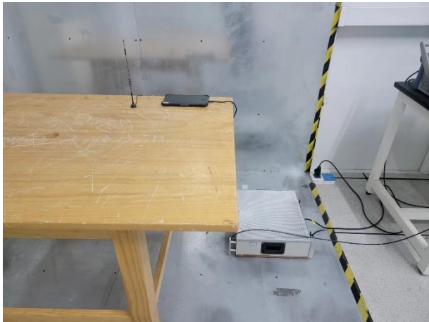
Radiated Emission test set-up for 30M-1GHz, TM1
